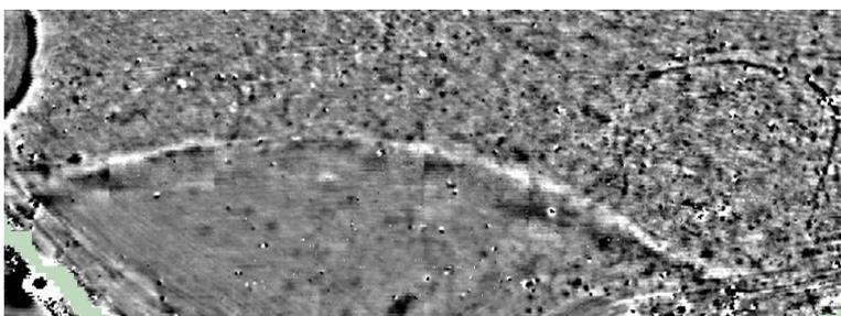
Traversal Destriping & clip at  $\pm 3SD$ . Destriping improves the appearance of the quiet area, allowing ploughmarks to show through. However, it has almost entirely removed the linear response where it runs parallel to the direction of survey. It also produces distinct disjunctions at grid edges.
