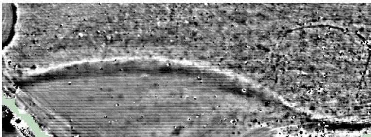
Processing is just clip at  $\pm 1SD$ . The long curving anomaly due to the terrace edge is clearly visible across the centre of the survey. However striping, especially in the relatively quiet area below the terrace feature, is severe.
