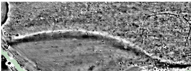
Sensor Destriping & clip at  $\pm 3SD$ . Now the linear anomaly remains intact and is almost identical to the raw version. There are only the slightest hints of grid edges and yet almost as much detail of the ploughmarks is visible in the quiet area.
